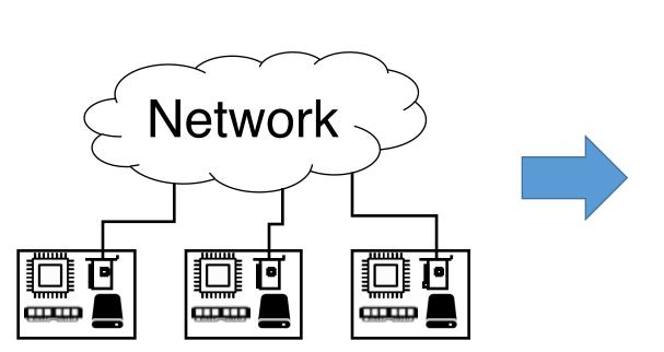
Server centric architecture: each server is a self-contained system comprise of CPU, memory, disk, and other peripherals
