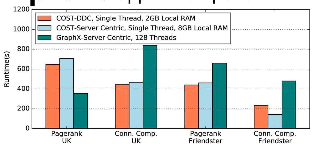
Applications can benefit from disaggregation by avoiding coordination and serialization overhead
